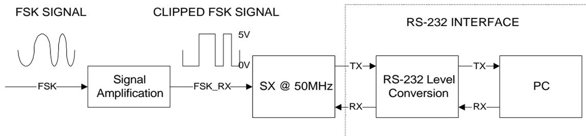
Demonstrating FSK detection requires this type of circuitry, in addition to some means of creating the FSK signal. Integrating this type of solution into an operational modem would require one additional block: the isolation circuitry, which isolates the outside phone line from the modem's internal analog circuitry. There are standard isolation circuits for every country, so check with the local standards committee.
